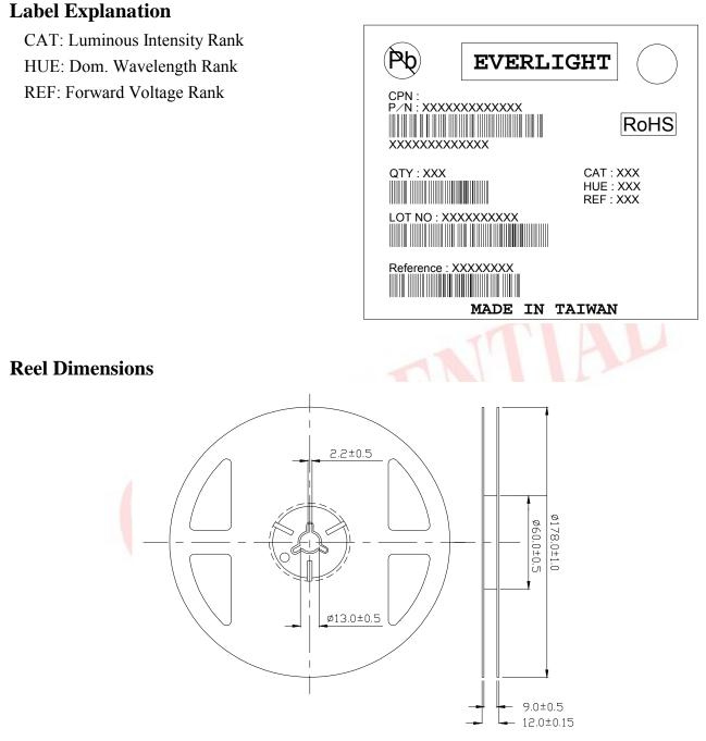
**Note:** The tolerances unless mentioned is  $\pm 0.1$  mm ,Unit = mm
