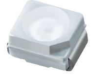
• The 67-21 series is available in soft orange, green, blue and yellow. Due to the package design, the LED has wide viewing angle and optimized light coupling by inter reflector. This feature makes the SMT TOP LED ideal for light pipe application. The low current requirement makes this device ideal for portable equipment or any other application where power is at a premium.
